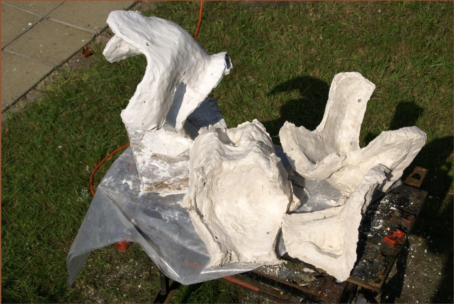
The 3 pieces of the plaster mold
