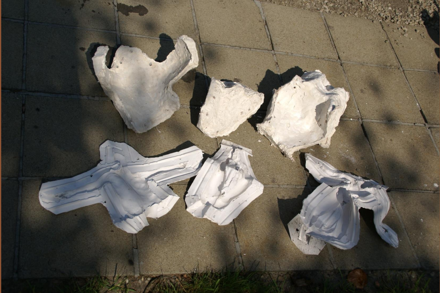
The parts of the rubber/plaster mold
