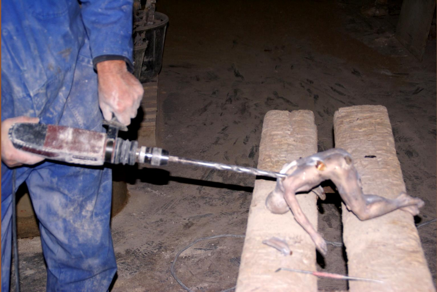
Removing the plaster inside
