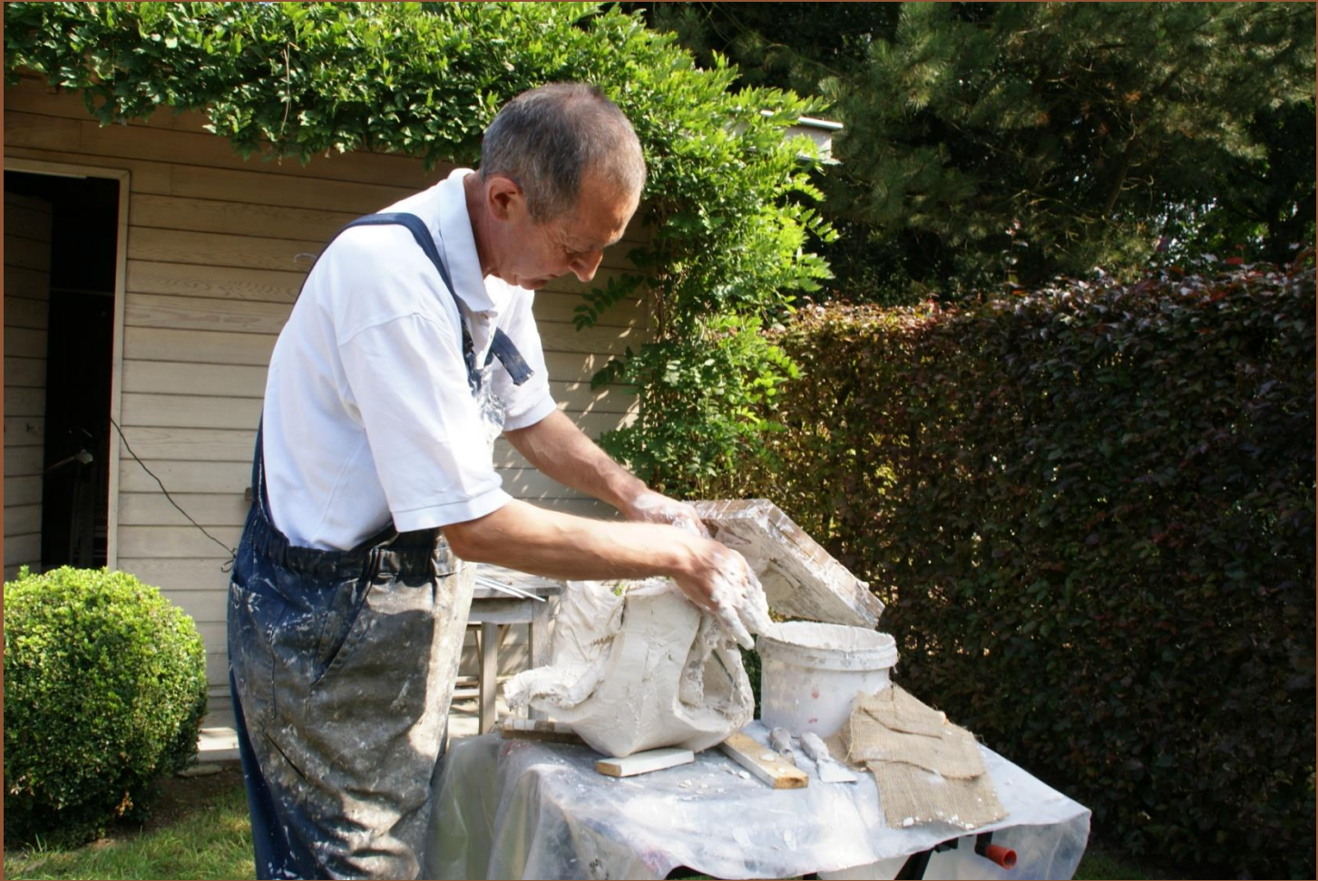
Making plaster mold on the rubber mold
