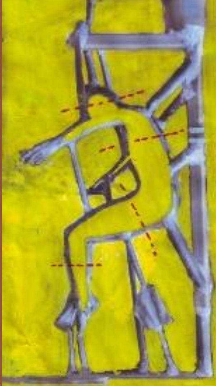
Intersection of the molding cilinder with the wax sculpture inside
