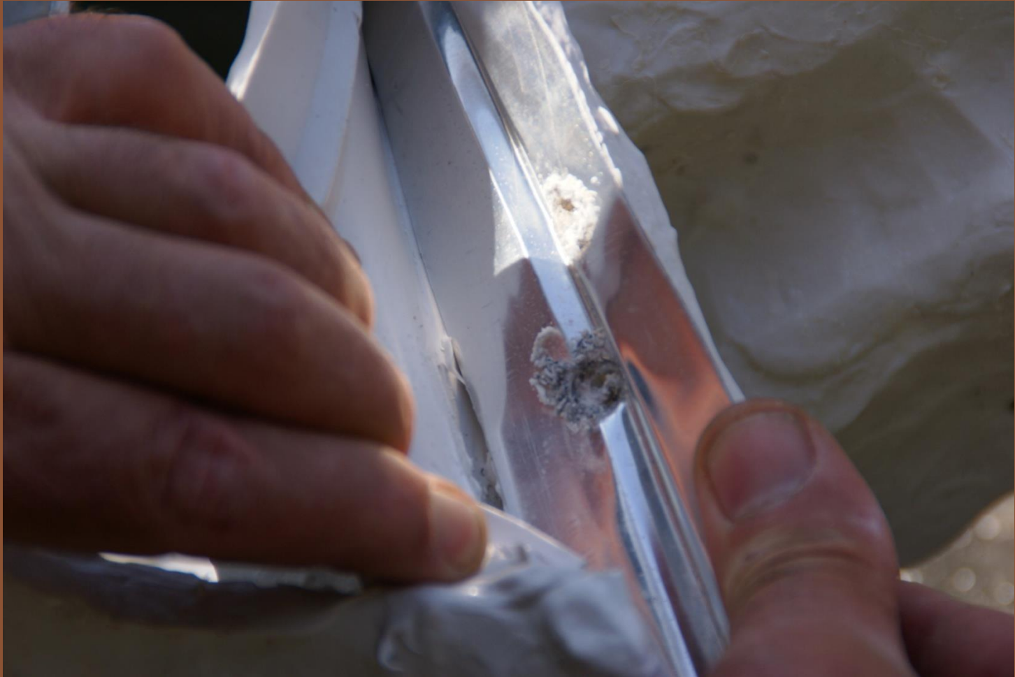
Unfasting the rubber mold
