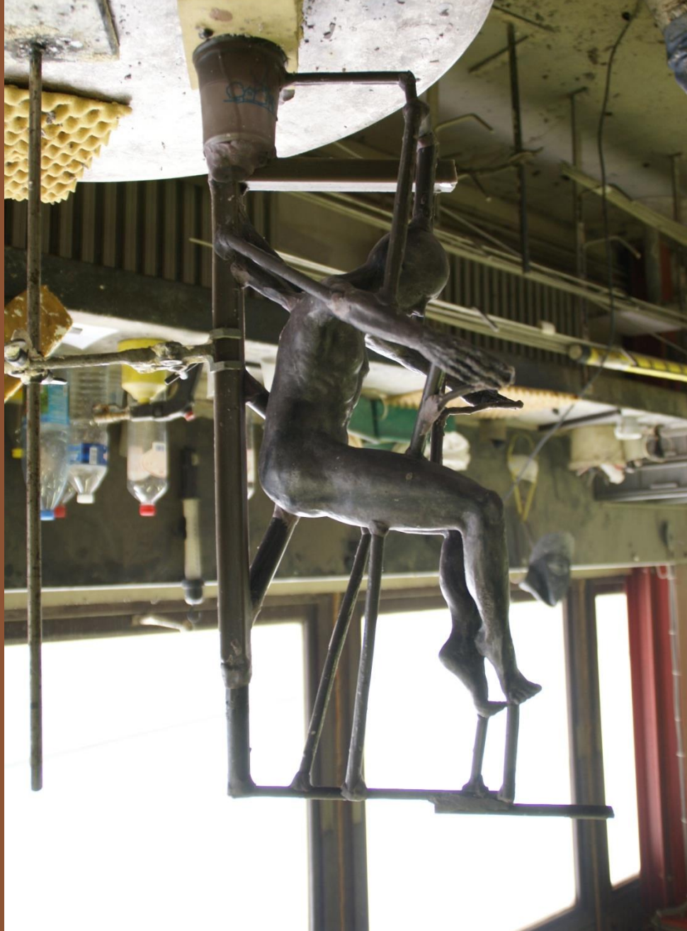
All elements in wax are mounted.
