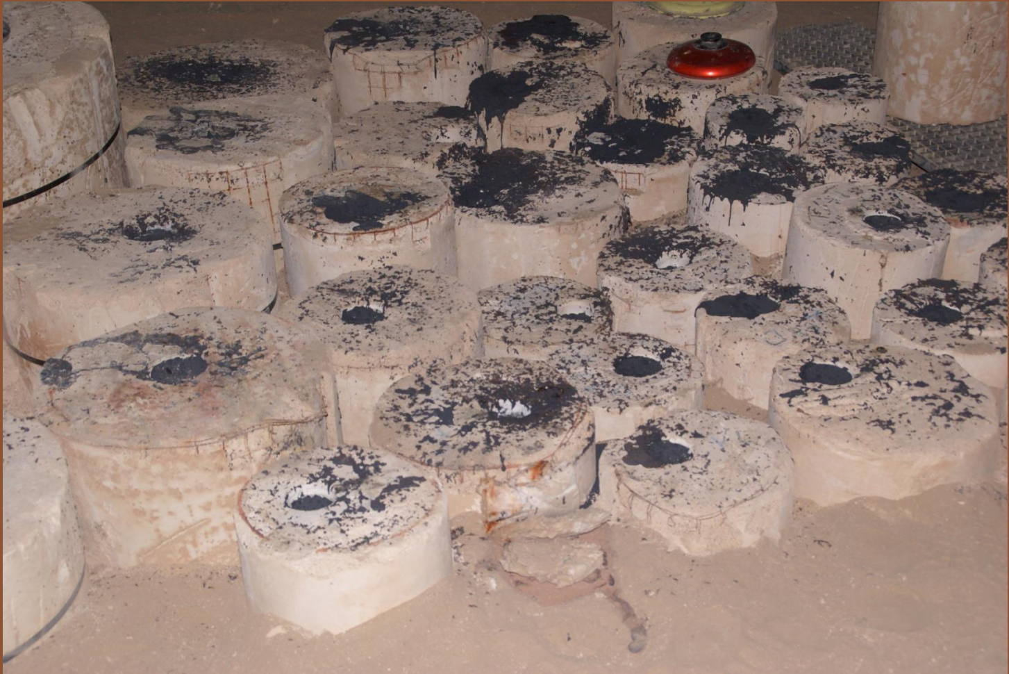
A few minutes after the casting ready to cool off for 3 days
