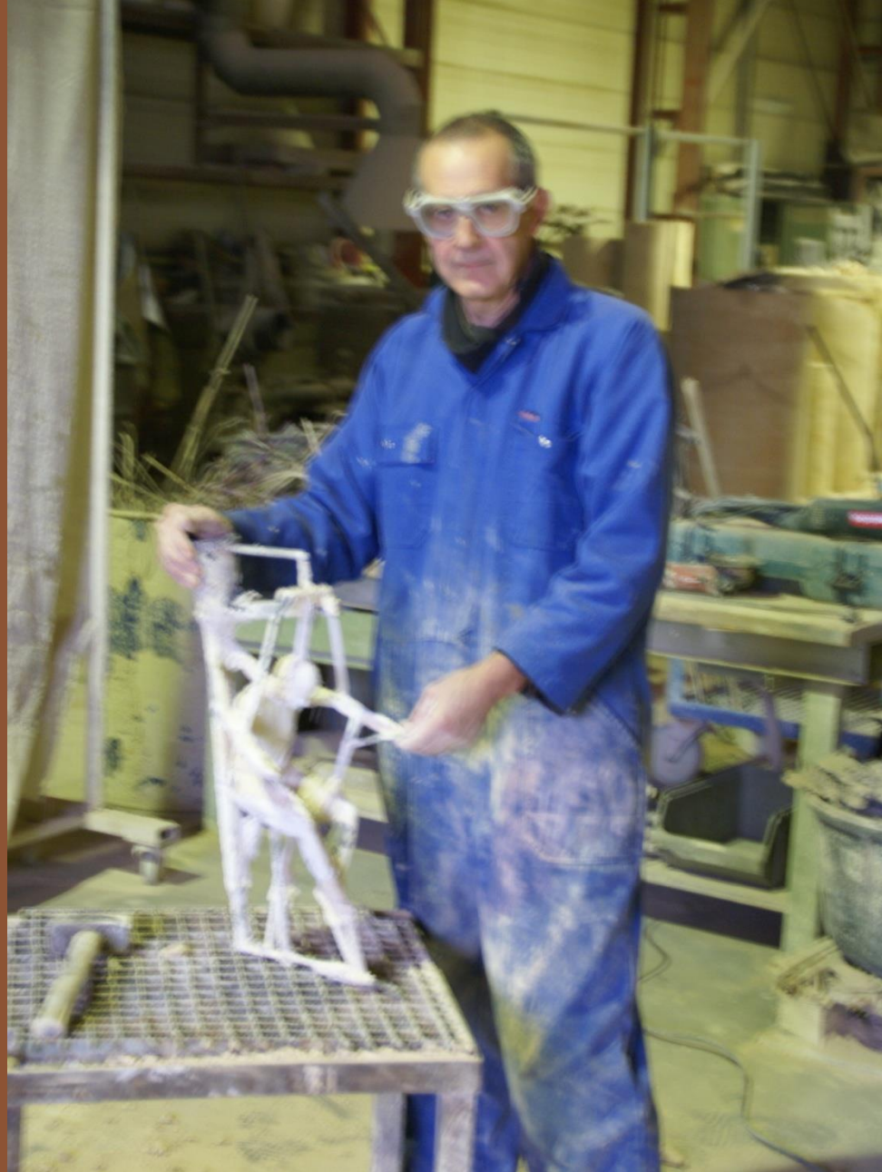
Bronze sculpture with casting pipes and plaster layer
