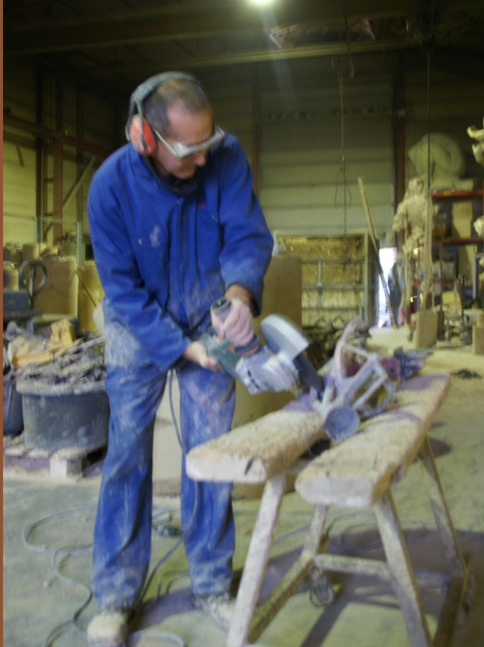
Cutting off the casting pipes
