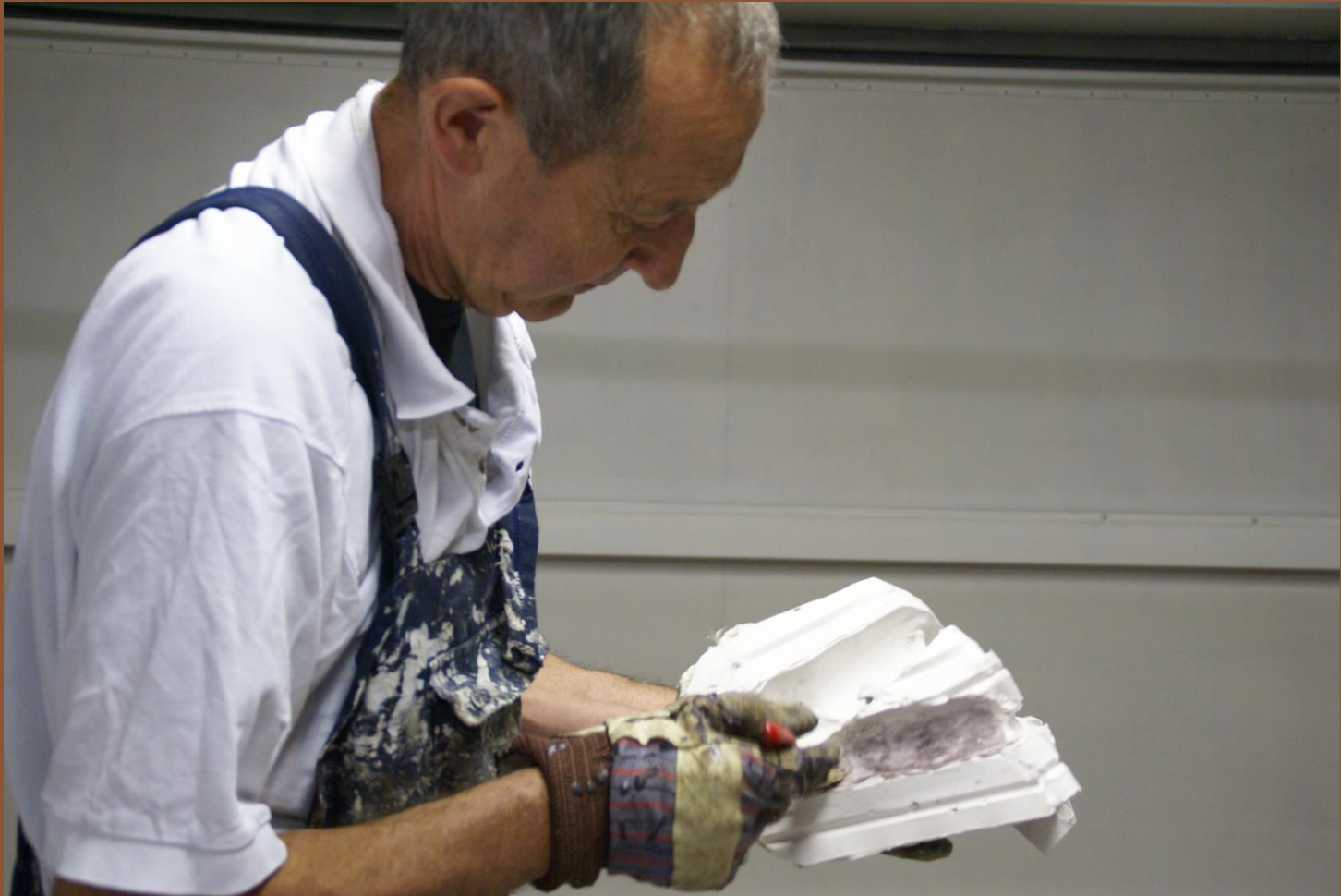
Brushing warm wax into the rubber mold
