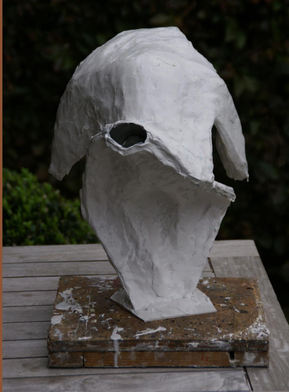
Opening in rubber mold used to pour in the wax
